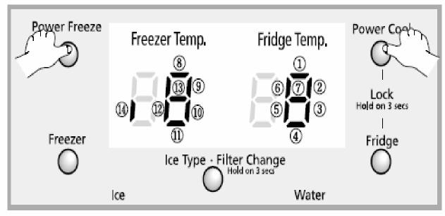
If any LCDs blink, the corresponding sensors and components must be checked for an error.
