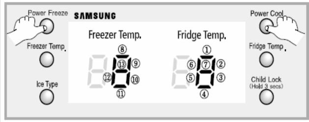
If any LEDs blink, the corresponding sensors and components must be checked for an error.
